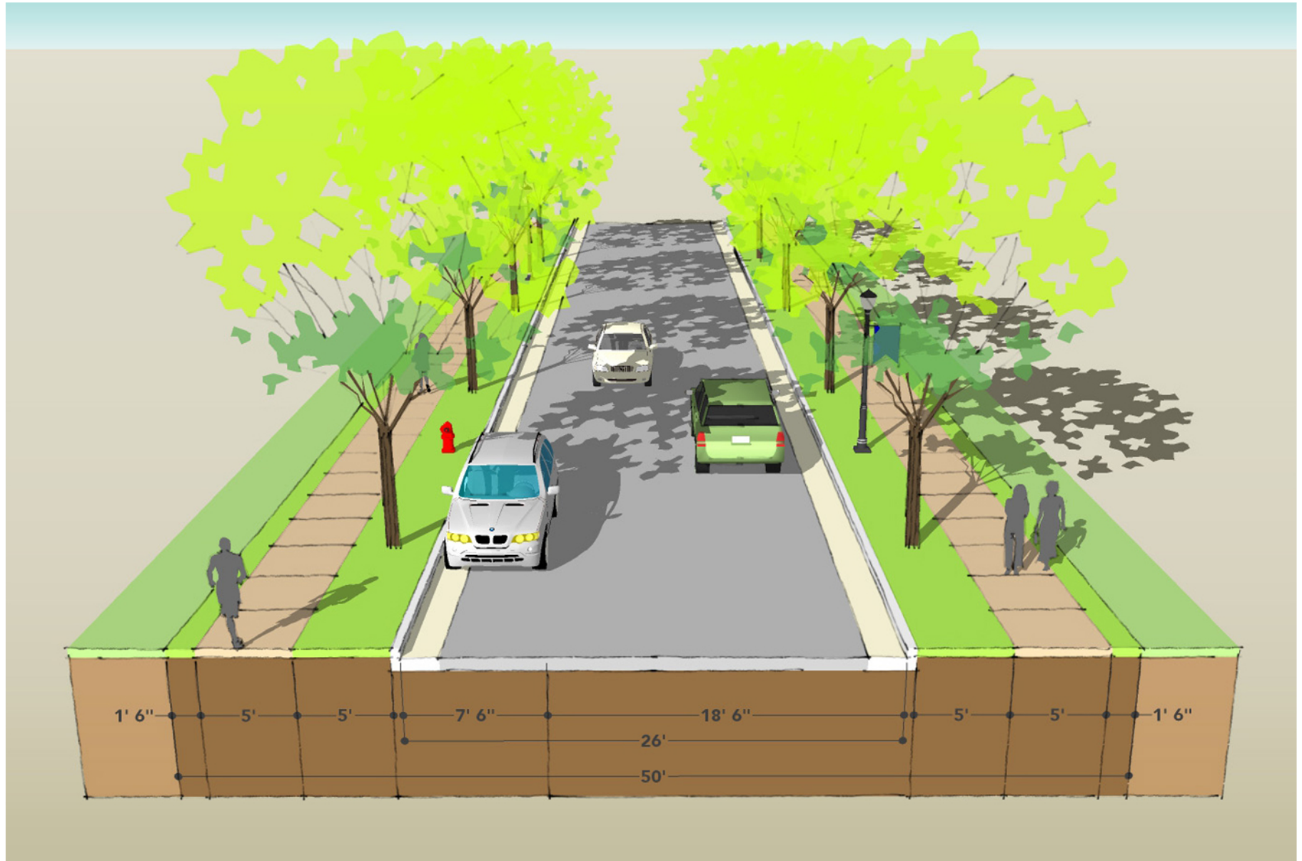
Potential streetscape enhancements to existing 50' ROW includes 5 feet wide sidewalks on both sides of the street allow two pedestrians to walk side by side comfortably. Street trees in a 5 feet tree lawn and decorative light fixtures define the street and help slow traffic. On-street parking on one side of the street still allows for 2-way traffic.
