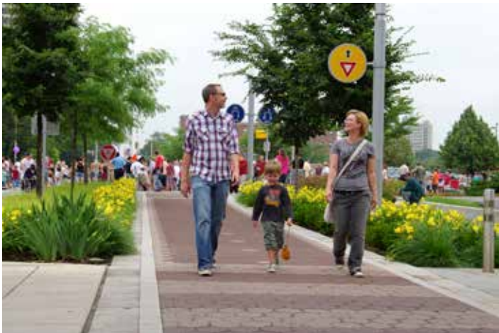
BUFFERED MULTI-USE TRAILS. LATERAL BUFFER PROVIDES ADDITIONAL SPACE BETWEEN AUTOMOTIVE AND PEDESTRIAN. SOURCE: MATT CARROLL, HTTP://INDYCULTURALTRAIL.ORG/ABOUT/
