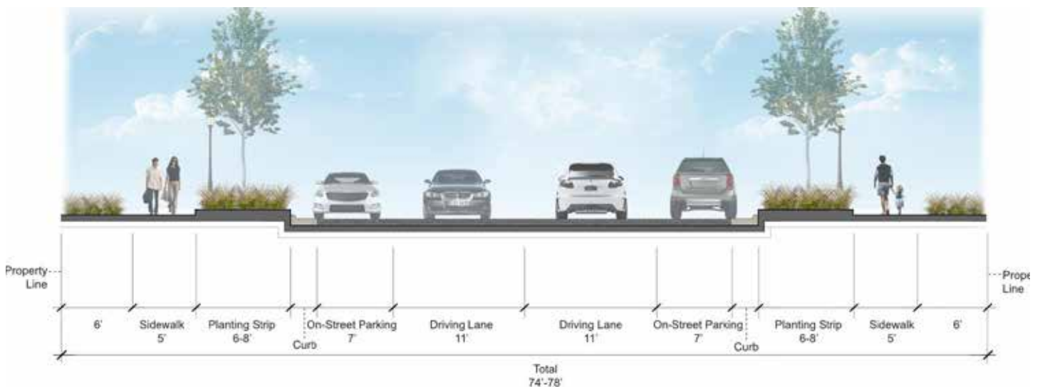
FIGURE 4.5: POTENTIAL CROSS-SECTION FOR RESIDENTIAL COLLECTOR STREET
