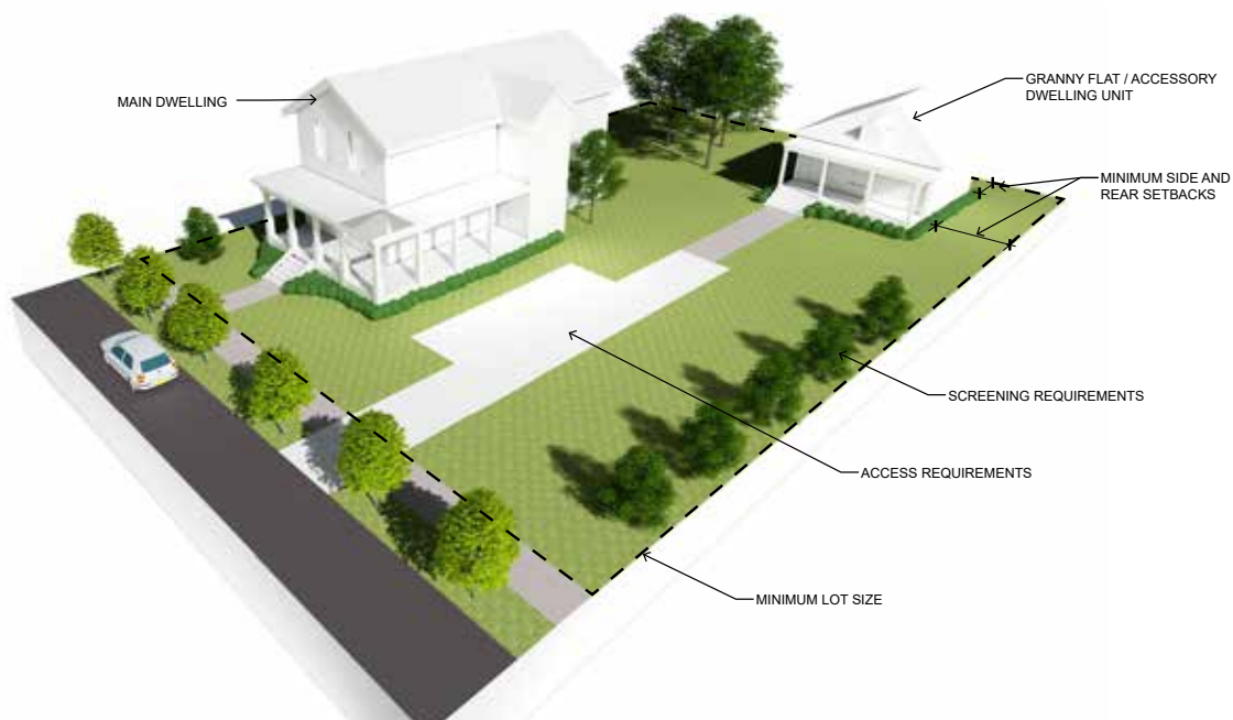
FIGURE 4.4: ALLOWING ACCESSORY DWELLING UNITS IN RESIDENTIAL AREAS COULD BE ONE WAY TO INCREASE HOUSING OPTIONS WHILE RETAINING THE RESIDENTIAL CHARACTER OF SOME PARTS OF OLD TOWN.
