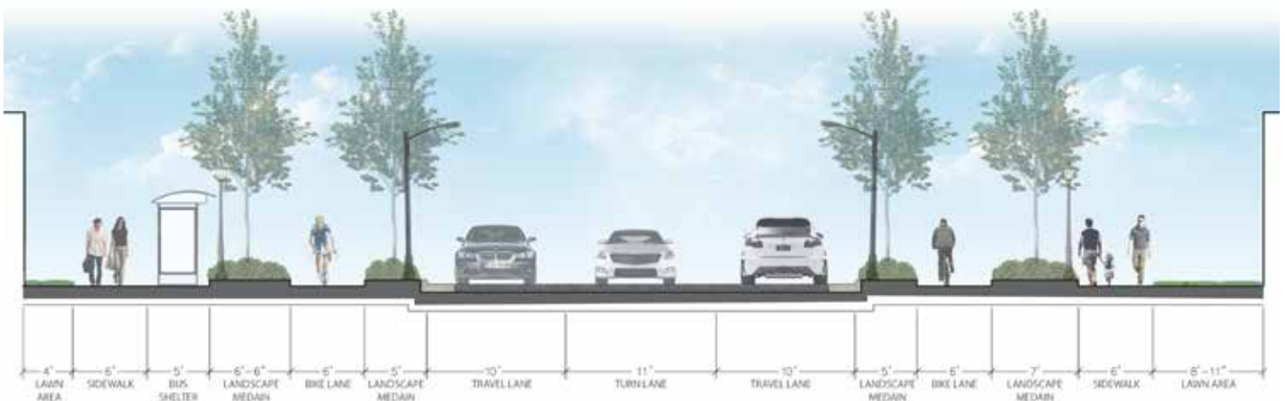
FIGURE 4.16: POTENTIAL CROSS-SECTION FOR 100' RIGHT-OF-WAY ROADWAY
