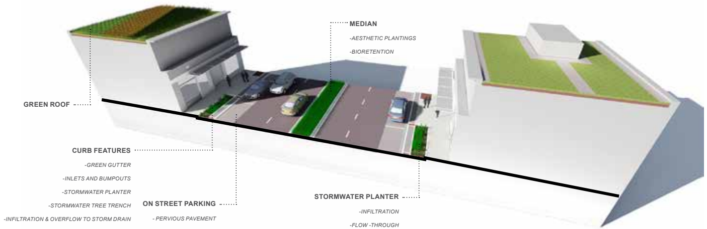
FIGURE 4.11: GREEN STREET LOW IMPACT DEVELOPMENT (LID) TECHNIQUES
